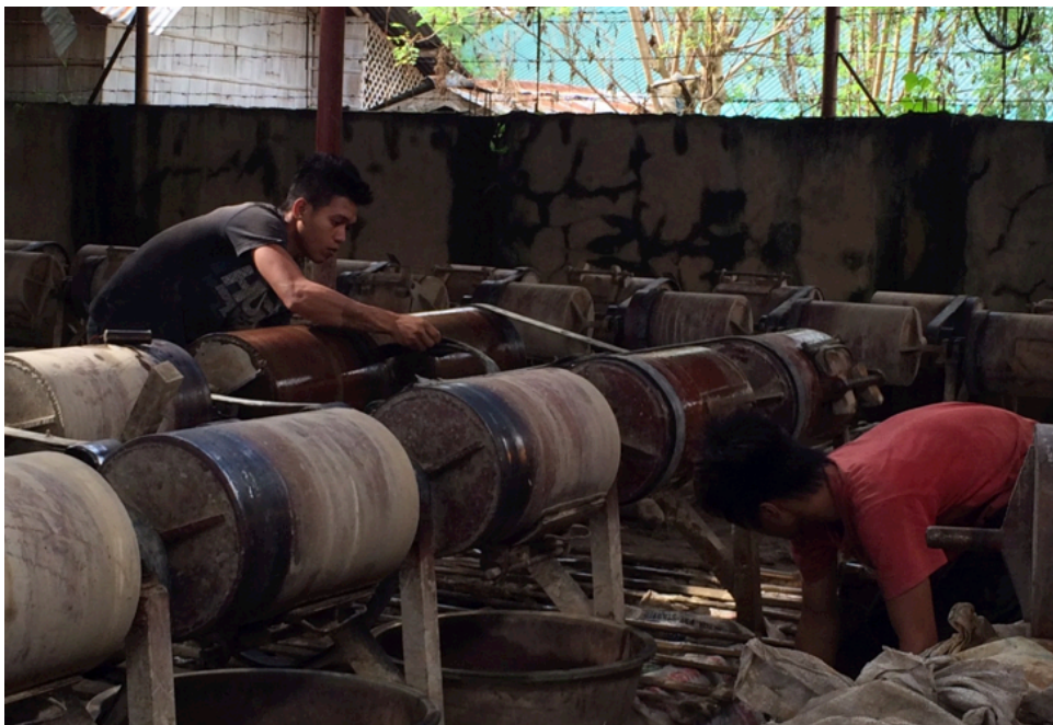
Small-scale mining in T’boli: Ore is pulverized in a drum machine to free gold from rock by using mercury.
